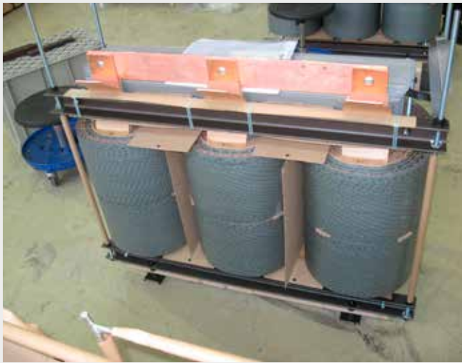
Figure 12. 1000 kVA / 24 kV prototype transformer, Končar D&ST, Croatia
