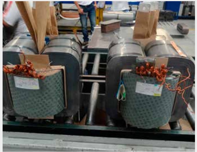
Figure 13. 75 kVA / 95 kV BIL transformers, MAGNETRON S.A.S, Colombia
