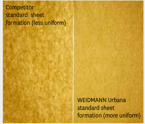
Figure 5. WEIDMANN and competitor paper formation (paper 0.76 mm / 3 mil; 0.75 g/cm 3 )
