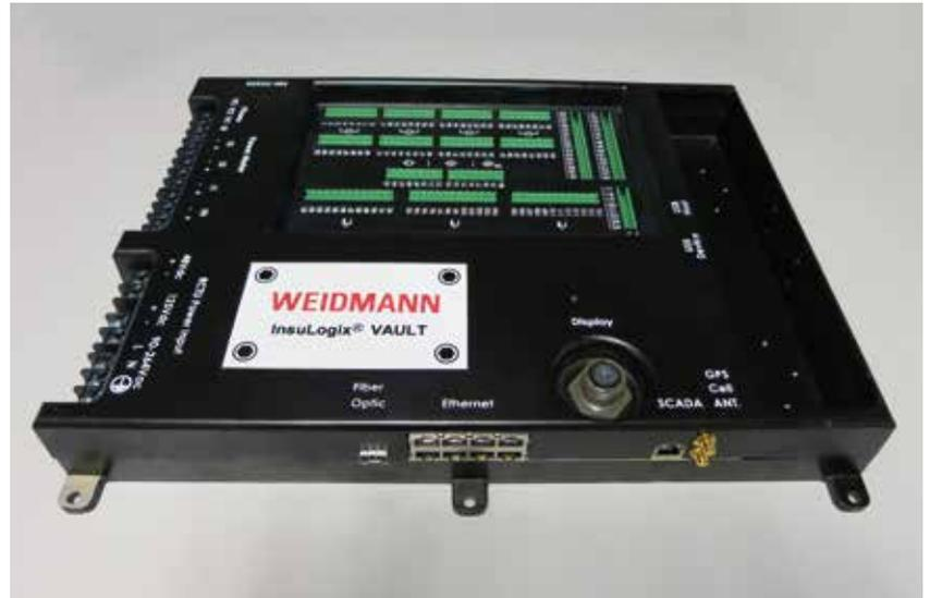
Remote Command Telemetry Unit (RCTU)
