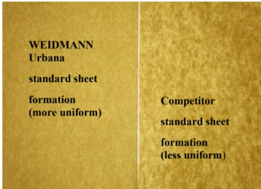
Fig. 2-10 Weidmann's and other manufacturer's paper formation (paper 0.76 mm, 0.75 g/cm 3 ).
